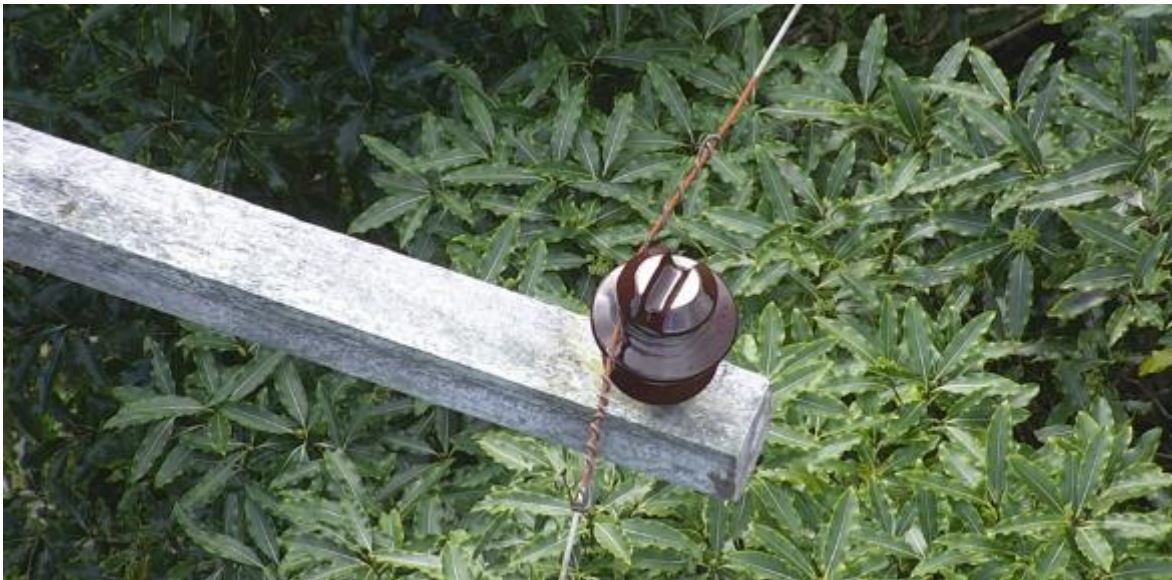
Figure 8.21: Rusty No. 8 wire at an insulated tie point due to bi-metallic corrosion
