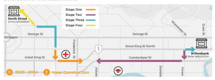
We are installing a new 2.5km 33 kV underground cable across Dunedin Central. The cable will run from Smith Street zone substation towards North Dunedin, to the Willowbank zone substation on Great King Street.
