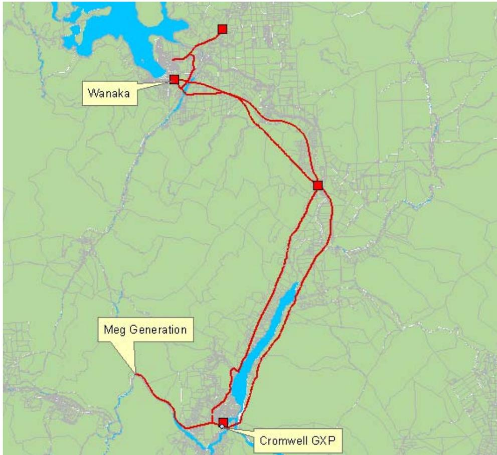
**Figure 3.5 - Cromwell Sub-Transmission Network**
