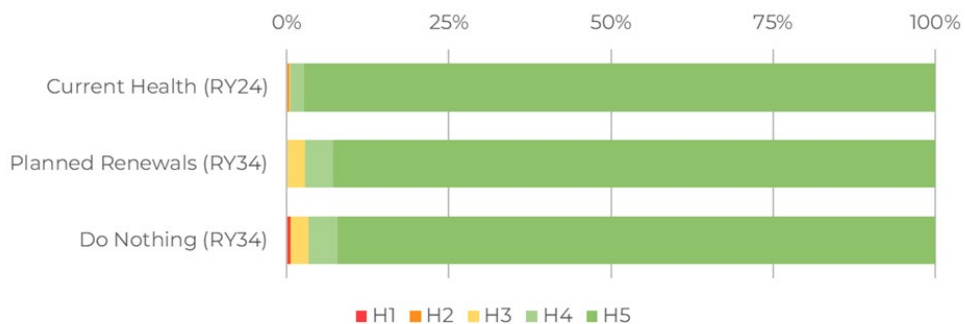
Figure 11-25: Projected distribution cable asset health
