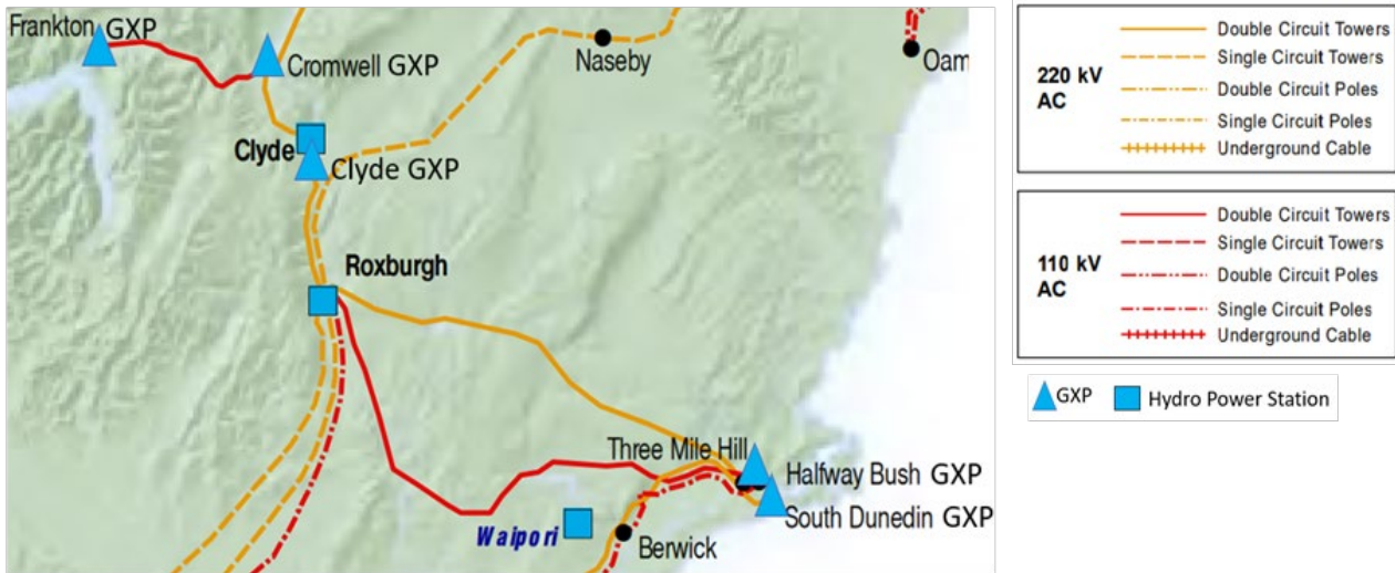
Figure 3-2: GXPs and transmission lines (map from Transpower)
